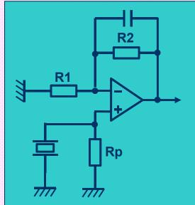
In a non-inverting voltage preamplifier, the equivalent input noise voltage spectral density is determined as follows (R1 << Req):
